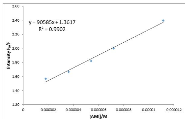
**Figure 9-** Stern Volmer plot of quenching of CRSA by Amisulpride
