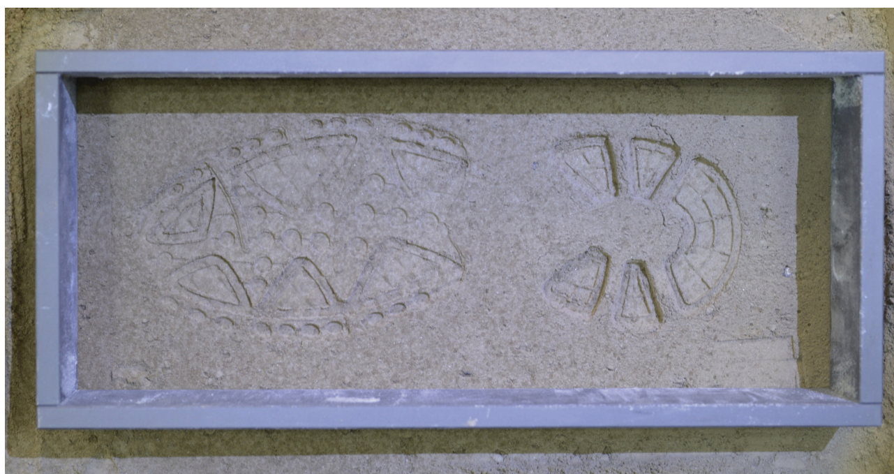
Figure 2 - The aluminum mold used for casing three-dimensional footwear impressions
