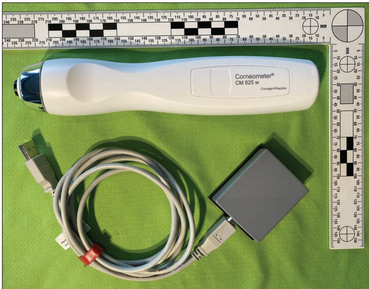
Figure 1- Photograph of the wireless version of the Corneometer CM-825®, accompanied by the device that must be connected
