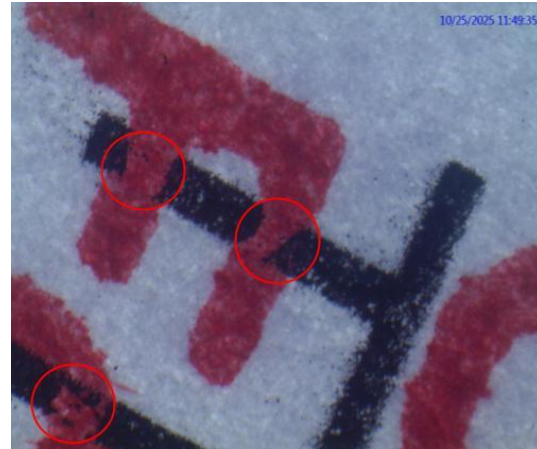
Figure 4- Gaps seen in toner layer when present above the stamp impression on standard A4 paper (magnification 1.25x)
