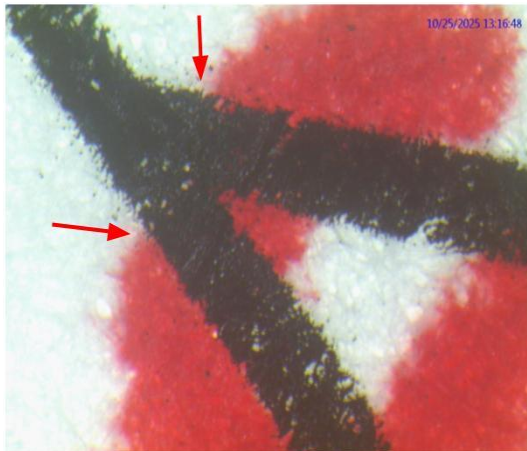
Figure 7- Narrowing of the stamp pad ink stroke when it is applied on top of the toner (magnification 2.5x)
