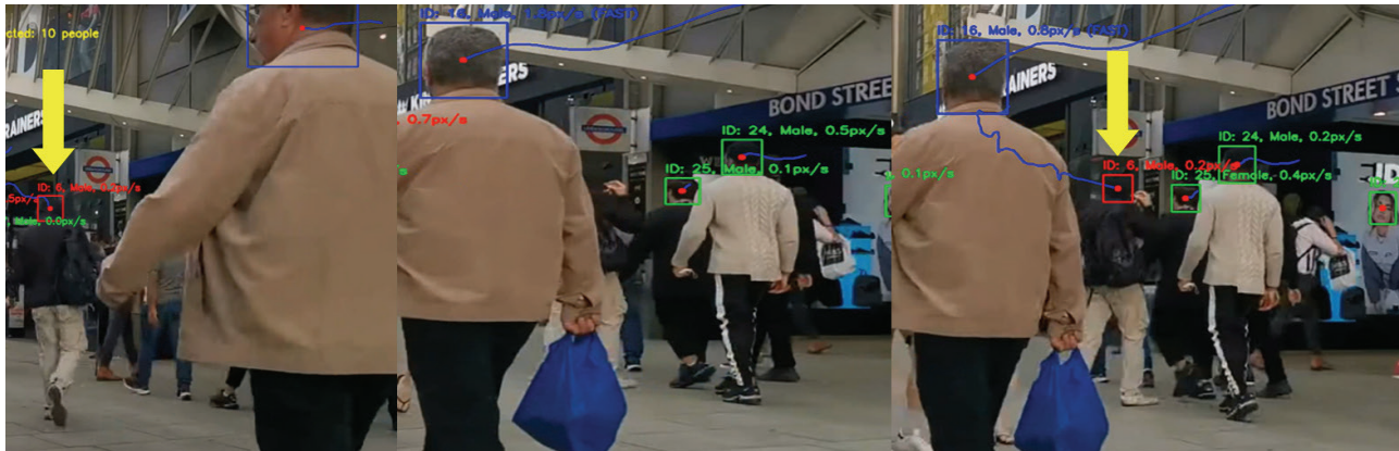
Fig. 3. Demonstration of continuous tracking under occlusion. A man (shown under a yellow arrow, left) is occluded (middle) and then reappears (right), with the same ID number.
