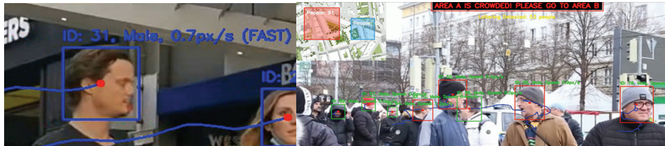
Fig. 5. Detection of abnormal speed (left) and surge detection near an event gate (right).
