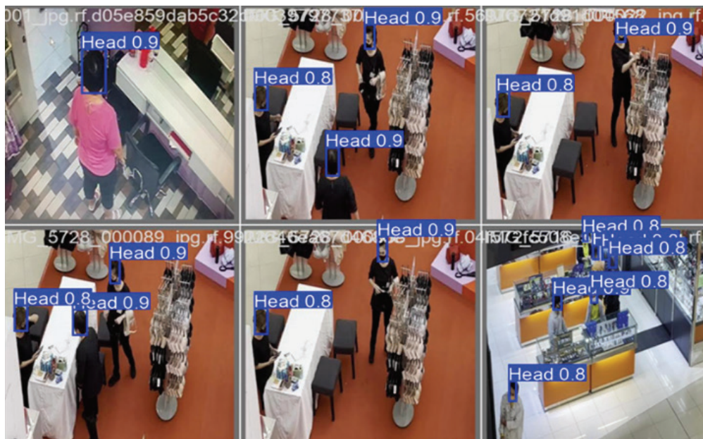
Fig. 2. Real-time head detection example using a public dataset in a shopping mall environment
