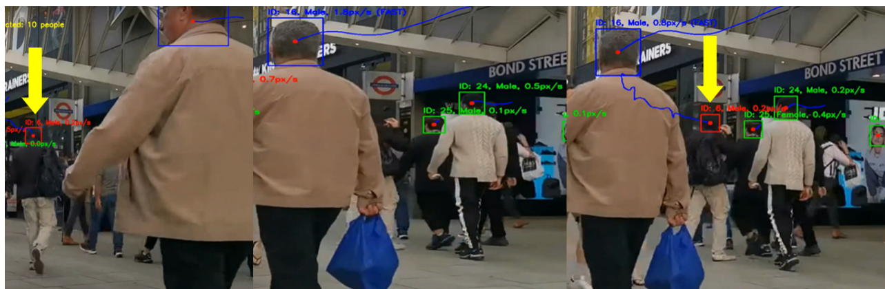
Fig. 3. Demonstration of continuous tracking under occlusion. A man (shown under a yellow arrow, left) is occluded (middle) and then reappears (right), with the same ID number.
