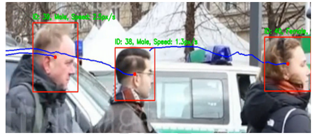
Fig. 4. Real-time gender classification (in green label over the bounding boxes) using custom-collected datasets.
